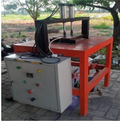
Gambar 4. Mesin Hot Press
